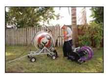
important feature that allows LMK's Performance Liner® to be visually inspected by CCTV before the
