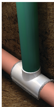
Figure 1: Outside Sewer Service Cleanout through a Minimally Invasive Small Bore Vacuum Excavation
