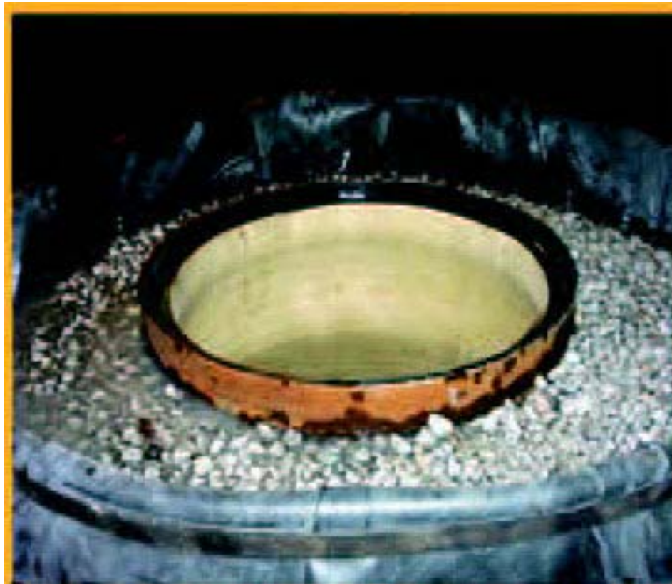
Picture 3. Manhole Test Assembly with Flooded Backfill
