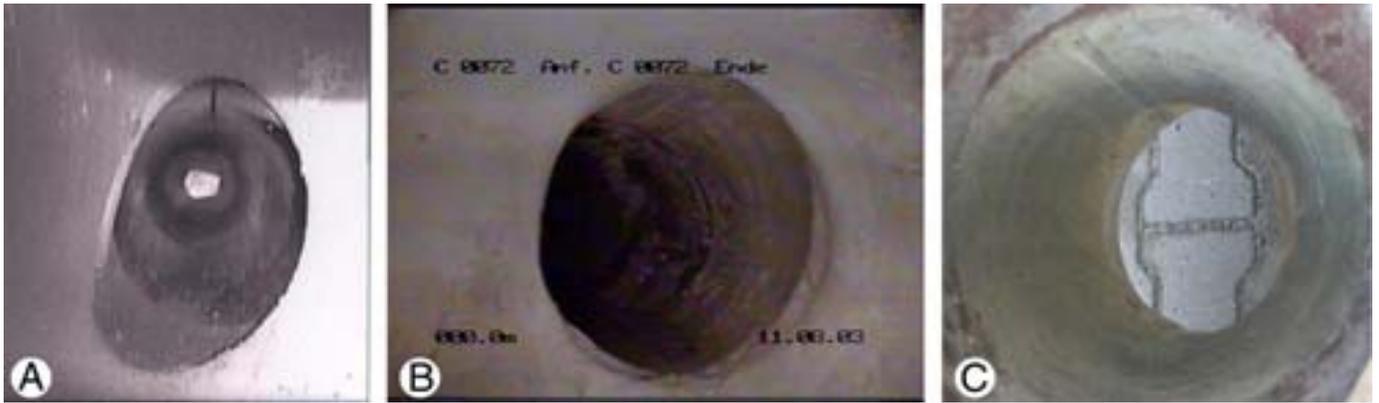
Figure 5. Extreme damage for top hat liners and example of a visually satisfactory repair result. **A** Initial situation. **B** View from the main pipe. **C** View into the connecting pipe (after disassembly).
