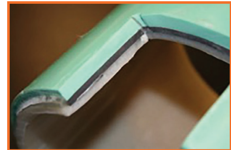
RIGHT: PVC pipe with Insignia End Seal Gasket installed at terminating end of CIPP liner.
