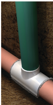
Figure 1: Outside Sewer Service Cleanout through a Minimally Invasive Small Bore Vacuum Excavation
