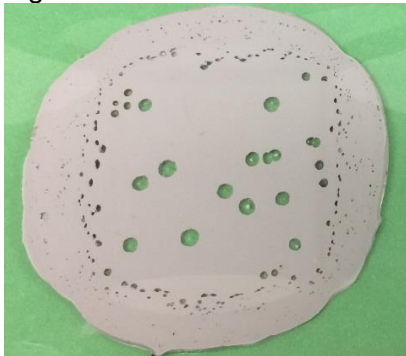
Figure 12: Shrinkage voids in a P-201A sample after 20psi compression in Melinex releasing paper after 10 days of curing.
