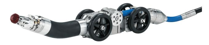
High-pressure water technology MICROcleaner up to 1000 bar (DN 100 - 200 / 4" - 8")
