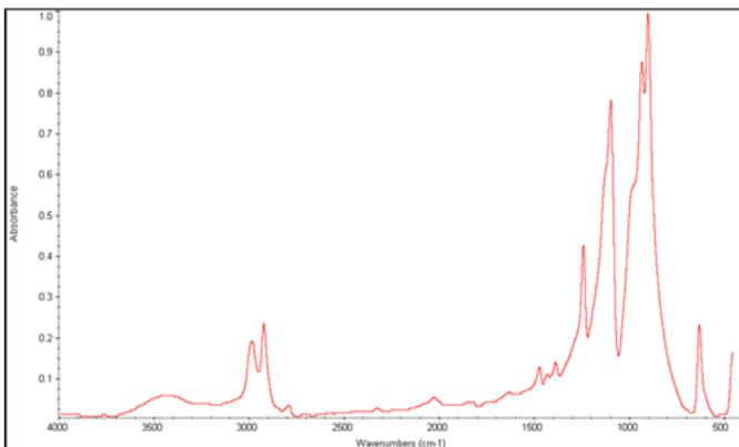
Fourier Transform Infrared Spectroscopy (FTIR) Resin Fingerprint
