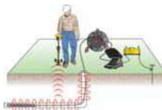
Find plastic pipe by tracing the push cable
