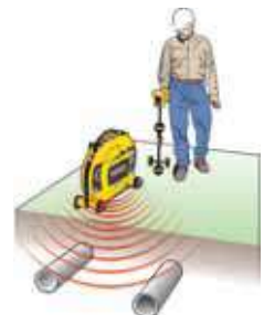
Induce a signal to locate utilities.
