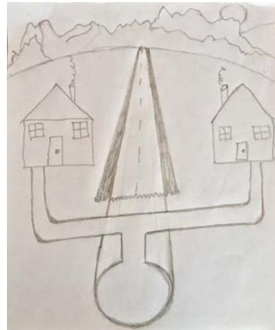
Fig 3. Double Tee Stack Connections
